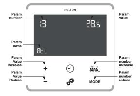
To leave the Settings mode to go to the main display mode press and hold the & key for 3
