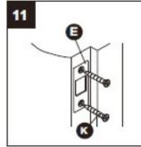
Install Touchpad Assembly Make sure the latch bolt is retracted.
